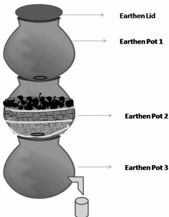
The technique for making pot shaped matka filter is similar to that of molding spindle shaped pots. The only difference is that for molding this only clay is mixed with sand in a 1:5 proportion (one part sand, five parts clay). From a trailer load of clay 500 pots of the dimension illustrated in Figure 3 can be made. This constitutes the outer body of the pot shaped matka filter.
