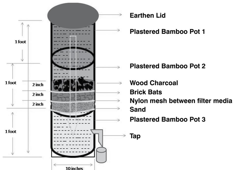
The hollow spindle like design of the bamboo matka filter is similar to the regular matka filter. The arrangement and working is also similar. The containers made of bamboo are plastered with a layer of cement and sand mixed in 1:3 proportions. After this the entire body is painted. The dimensions of this filter are- inner diameter of 10 inches, height 1 foot 2 inches and has a capacity of 24 liters. The cost of production of this filter is Rs. 550/-.
